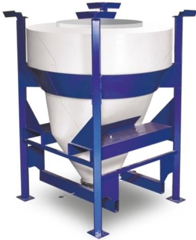
CPX Silos have a special design that enables mass flow, which facilitates container emptying. A slide valve is available as an accessory in both stainless steel and hot dip galvanised versions. However, the outlet can be modified as necessary and supplied both threaded and with a flange. The stand can be fitted with wheels and customised. Ideally, the stand is moved by means of a forklift. Also available in 1,200 L and 1,500 L versions.
