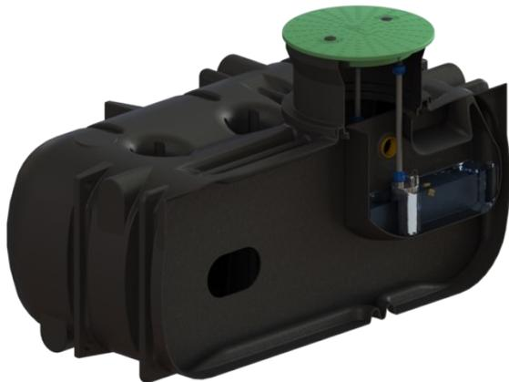
Robust, low buildt septic tank with large sedimentation volume and 3 chambers that provide an extra long sedimentation distance. The separation capacity is very high (0,06g). The flexible, robust design makes CPX Septic tank suitable for most ground conditions and allows the in- and out lets to be placed on both short and long sides of the septic tank.
