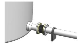
Installation of connections must be done with care so as to obtain a sealed connection without risking damage to the connection, gasket, or container/tank from excessive force. Lubricate the thread and gasket with a suitable lubricant (Silicone, PFPE) before tightening.
