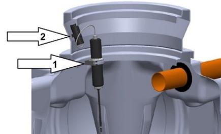
Drill a 16 mm hole for the cable entry. Burr the hole! Using an awl or similar, make a hole in the cable entry through which the cable is threaded.
